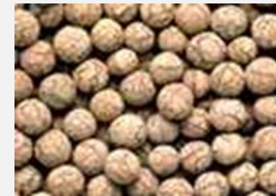
Biofilm on Filtration Material
